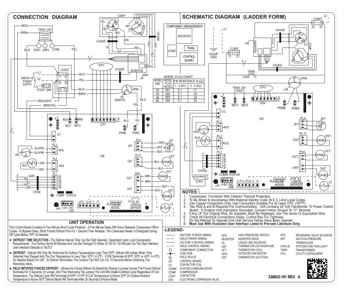
Fig. 1 – Wiring Diagram — Model sizes 2 – 5 tons, 208/230-1
