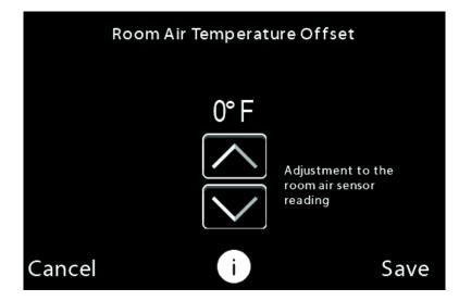
**NOTE**: Temperature sensors used in modern thermostats have defined tolerance intervals of normal temperature readings. This means if multiple of the same thermostat model were installed side-by-side, it would be normal for different current temperatures to be displayed (e.g. one at 72°F and one at 71°F). However, there are product features and installation steps you can take to help ensure a comfortable environment.
