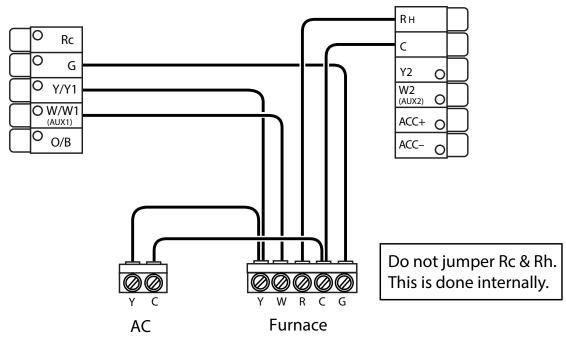
Two-Stage Furnace or Fan Coil with Single or Two-Stage A/C
