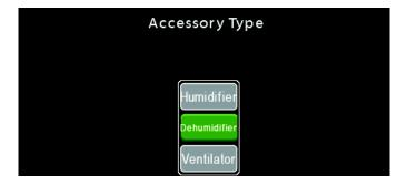
**NOTE**: The DHUM on fan coil board is active in the open state. The ACC+ terminal for dehumidifiers is defaulted to active open. So, no other changes are necessary. You can double check this setting on the thermostat:
