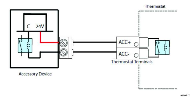
Per the diagram above, the accessory is self-powered. During the Guided Setup process, you can configure the accessory power source. When you select No, the internal relay on the thermostat will open.
