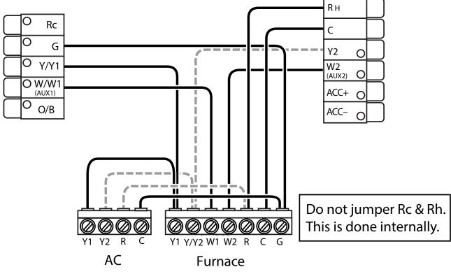
Two-Stage Heat Pump with Two stages of Aux Heat
