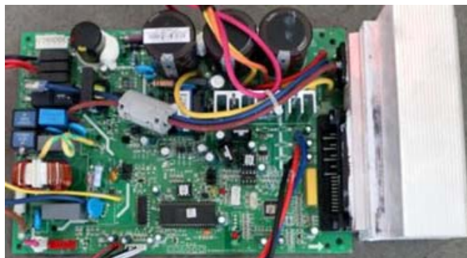
Fig. 28 – Outdoor (18K model) PCB
