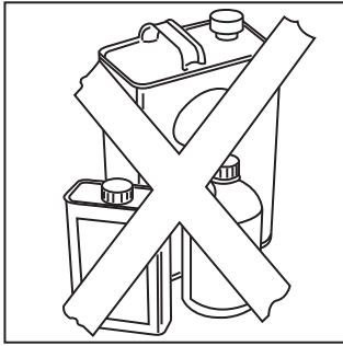
Fig. 4 - NO combustible materials near furnace
