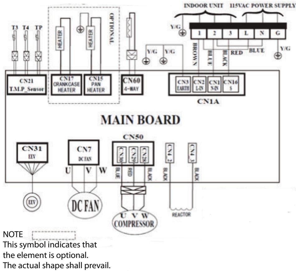
**Fig. 14 — Wiring Diagram Size 18K (208/230V)**
