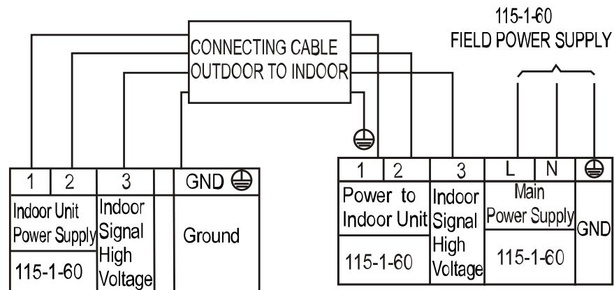
**Fig. 10 —Connection Diagram 12K (115V)**
