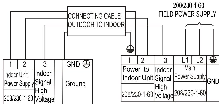
Fig. 11 —Connection Diagram Sizes 6K-36K (208/230-1-60V)
