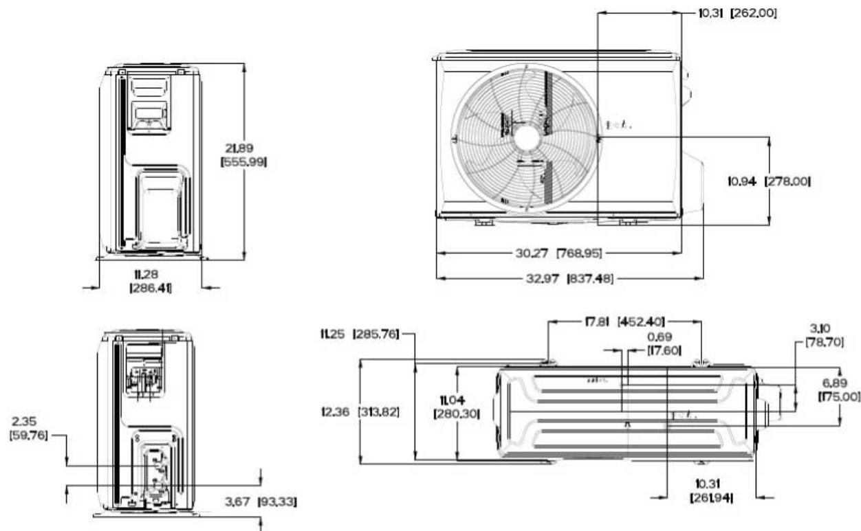
Fig. 3 —Dimension Sizes 12K (115V) and 6K (208/230V)
