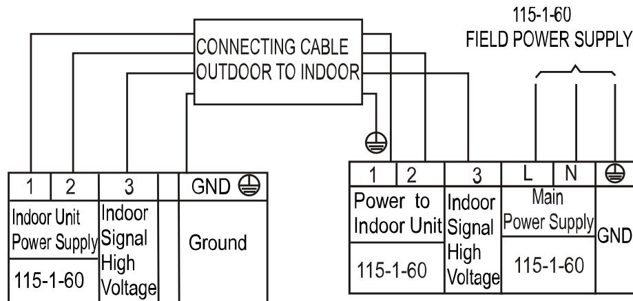
Fig. 10 —Connection Diagram 12K (115V)
