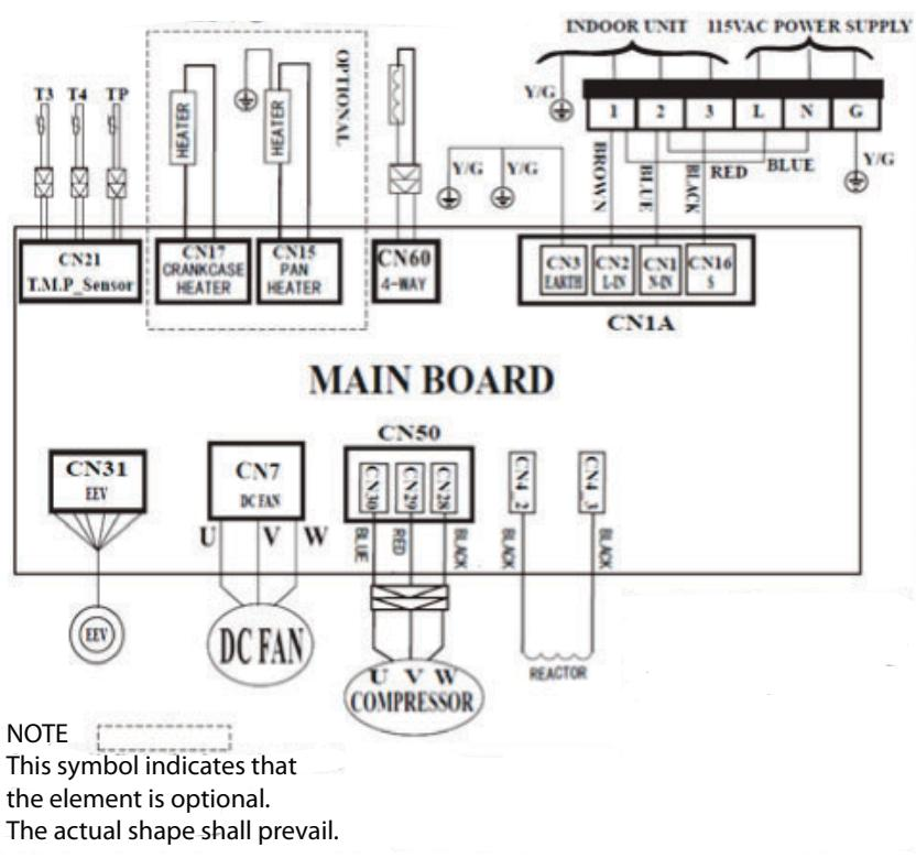
Fig. 14 —Wiring Diagram Size 18K (208/230V)
