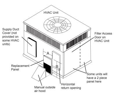
Fig. 1 - Hood Installation - Vertical Application
