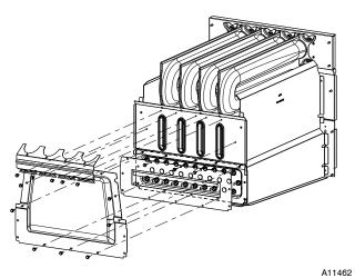
Fig. 6 - Coupling Box Cover & Finger Baffle Removal /
