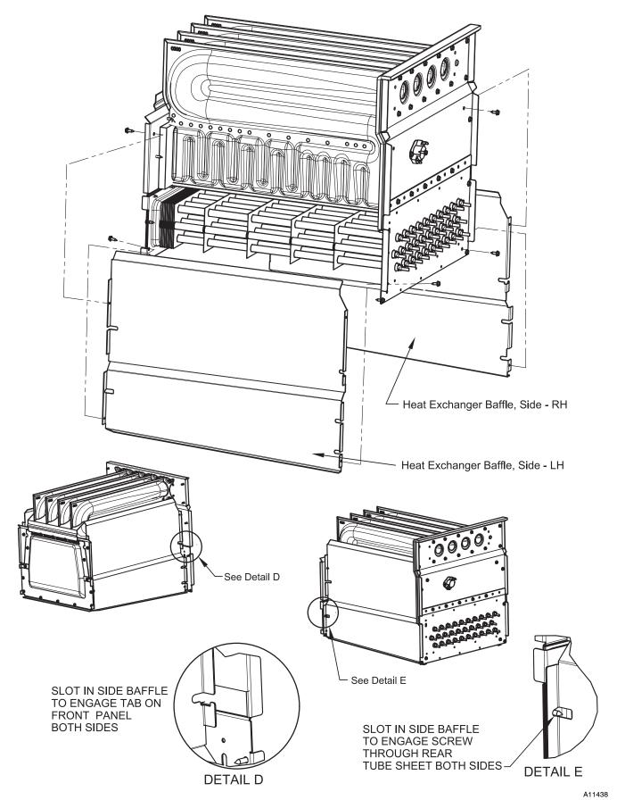
Fig. 9 - Heat Exchanger Panel Assembly
