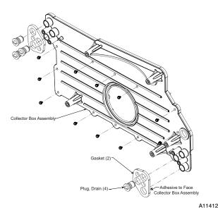
Fig. 5 - Collector Box Removal / Installation
