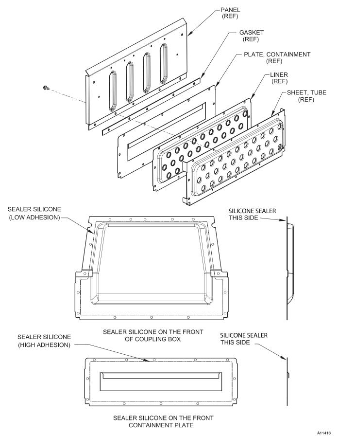
Fig. 10 - Containment Plate and Collector Box Sealant Application
