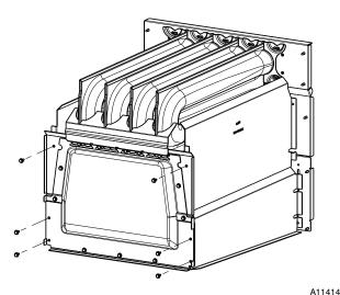
Fig. 7 - Sidewall Baffle Removal / Installation - Rear View
