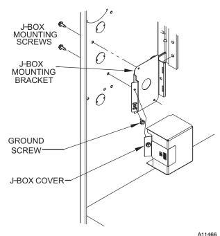
Fig. 4 - J-Box Removal / Installation
