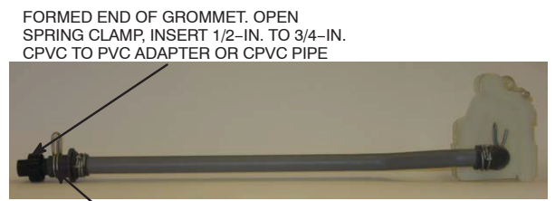
FRONT VIEW LEFT SIDE DRAIN PIPE ORIENTATION FOR CONDENSATE DISCHARGE NOTE: Remove Inducer Housing for easier access, if desired.
