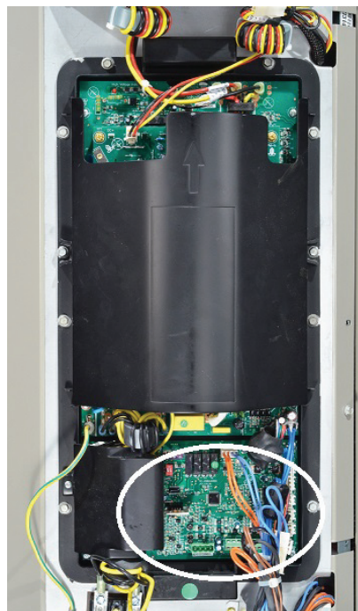
Figure 34 – Panneau de commande AOC (Application Operational Control)
