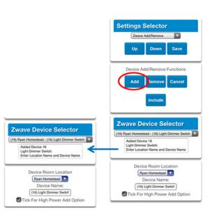
**Inclusion** can be used with a Z-Wave® remote Controller to assist with the **Add Device** process.
