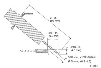
Fig. 10 - Igniter Position - Side View
