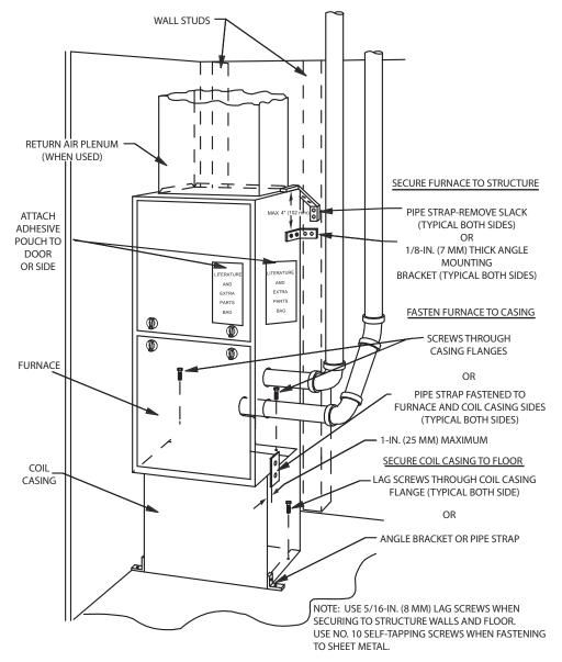
Fig. 1 – Securing Furnace to Structure
