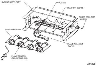
Fig. 5 - Burner Assembly
