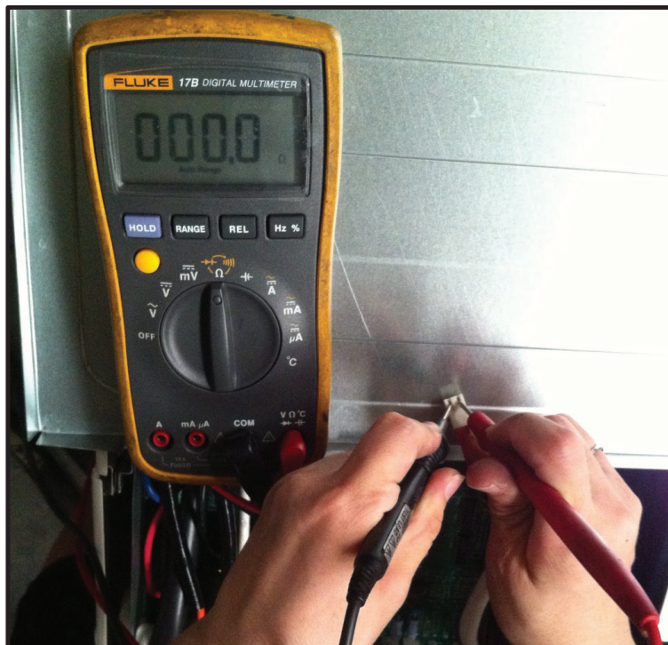
Fig. 59 – Test the resistance of the OLP
