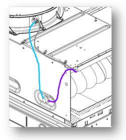
5. Using the 24 inch jumper wire, connect the fan stator limit switch to the leaving air temperature limit switch.
