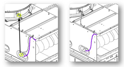
4. Take 24 inch piece of wire, strip ends, and crimp female connectors
