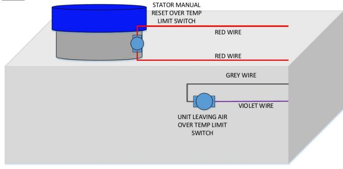
6. When completed, the wiring for the two limit switches should have changed as shown in the diagram below **Before:**
